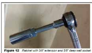
Figure 12 Ratchet with 3/8" extension and 5/8" deep well socket
