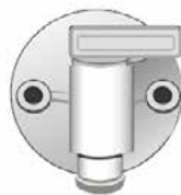
Exterior Fresh Water Drain
