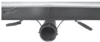
Black/Grey Tank Drain and Valves
