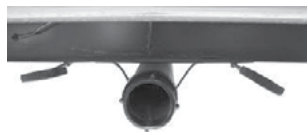
Black/Grey Tank Drain and Valves
