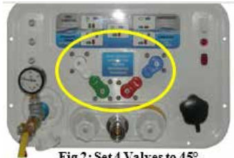
Fig 2: Set 4 Valves to 45°
