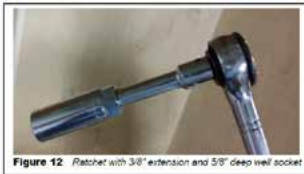
Figure 12 Ratchet with 3/8" extension and 5/8" deep well socket
