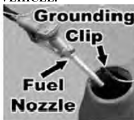
Fuel Nozzle in contact with receiving tank
