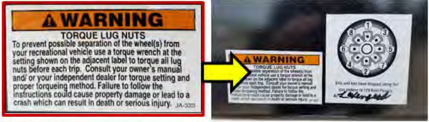
Lug nut torque pattern and warning label
