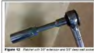
Figure 12 Ratchet with 3/8" extension and 5/8" deep well socket
