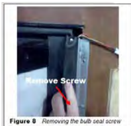
Figure 8 Removing the bulb seal screw
