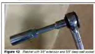
Figure 12 Ratchet with 3/8" extension and 5/8" deep well socket
