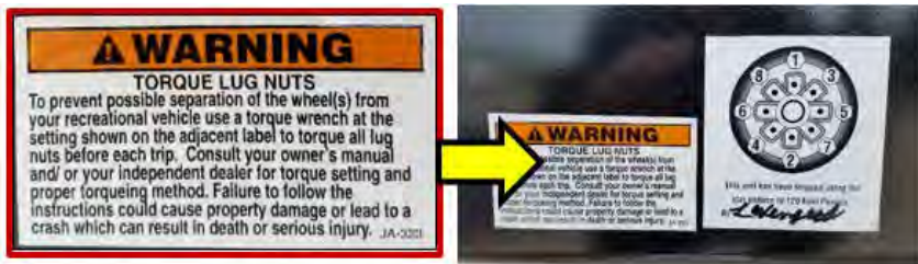
Lug nut torque pattern and warning label
