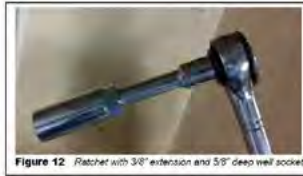
Figure 12 Ratchet with 3/8" extension and 5/8" deep well socket
