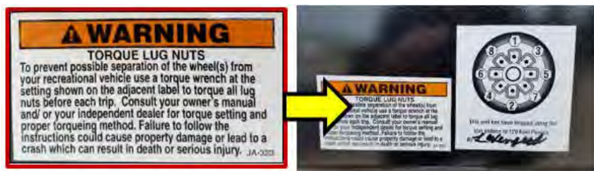
Lug nut torque pattern and warning label
