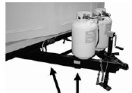
Electrical wiring & safety break-a-way switch Detachable Hitch
