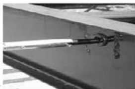
Fig. 2 - Through Frame Crank Extension w/Pin
