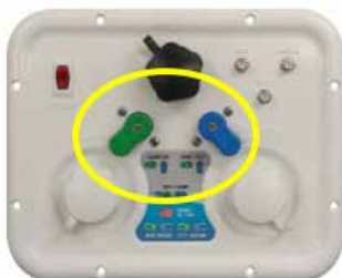
Fig 2: Set 2 Valves to 45°
