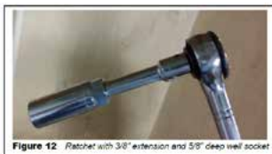
Figure 12 Ratchet with 3/8" extension and 5/8" deep well socket
