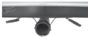
Black/Grey Tank Drain and Valves
