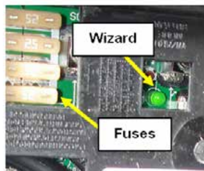
Wizard Button & Reverse Protection Fuses
