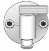
Exterior Fresh Water Drain
