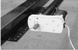
Fig. 3-Hex Head Crank Extension
