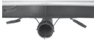
Black/Grey Tank Drain and Valves
