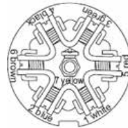
7-way trailer plug-rear view
