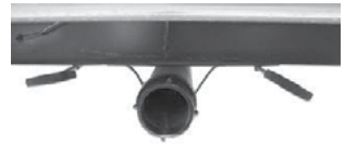
Black/Grey Tank Drain and Valves
