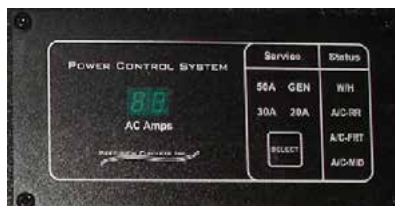
50A System Panel
