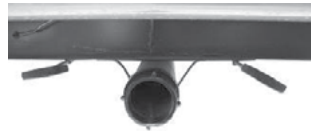
Black/Grey Tank Drain and Valves
