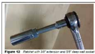
Figure 12 Ratchet with 3/8" extension and 5/8" deep well socket
