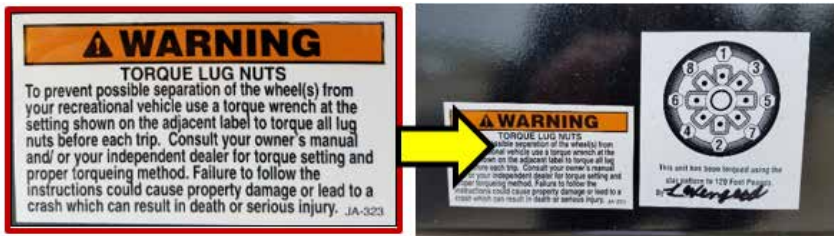
Lug nut torque pattern and warning label
