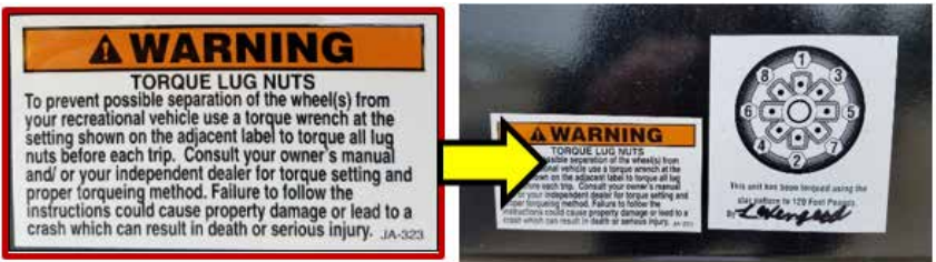
Lug nut torque pattern and warning label
