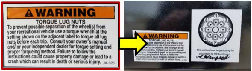
Lug nut torque pattern and warning label
