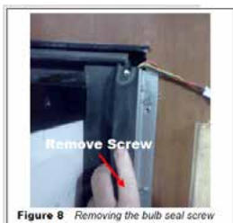
Figure 8 Removing the bulb seal screw
