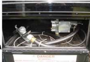
Master/Emergency Fuel Disconnect Switch locations
