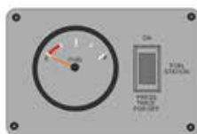
Single Tank Fuel Gauge and Selector
