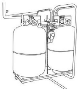
Two Propane Cylinders
