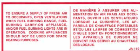
Ensure a supply of fresh air (Canada units only)
