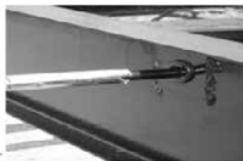
Fig. 2- Through Frame Crank Extension w/Pin
