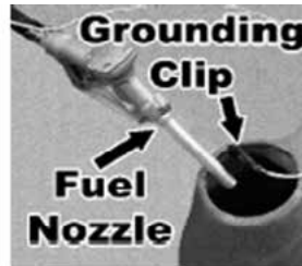
Fuel Nozzle in contact with receiving tank
