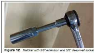
Figure 12 Ratchet with 3/8" extension and 5/8" deep well socket
