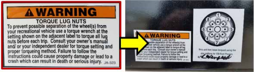
Lug nut torque pattern and warning label
