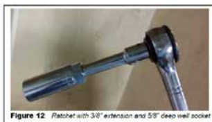
Figure 12 Ratchet with 3/8" extension and 5/8" deep well socket
