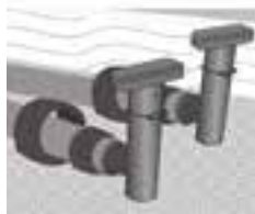
Low Point Drains
