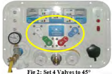
Fig 2: Set 4 Valves to 45°
