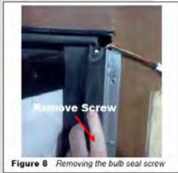
Figure 8 Removing the bulb seal screw
