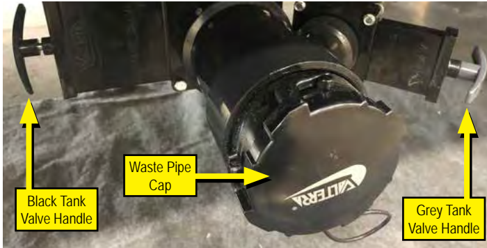
Example of Tank Drain Located Underneath RV
