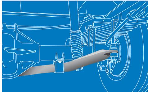
Reduces the body roll of a vehicle during fast cornering or over road irregularities
