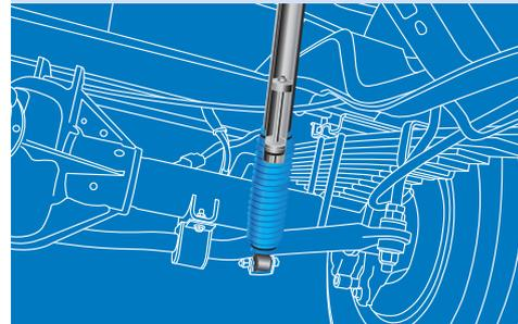
Feature a unique monotube gas-pressure design that provides optimum ride quality and vehicle control: Bilstein shock absorbers last 2-3 times longer than the conventional twin-tube piston and are found in many high-end luxury vehicles
