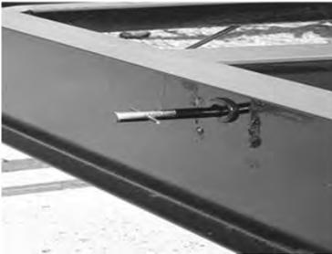
Fig. 1 Through Frame Crank Extension w/pin
