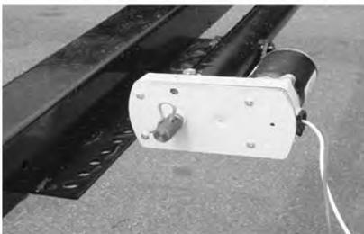
Fig. 3 Hex Head Crank Extension
