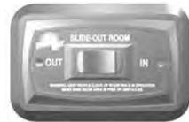
6. Release the switch, which will lock the room into position. If the slideout switch is held after the room is fully extended, the control will sense that the room has stopped and will shut the motor off after a few seconds.
