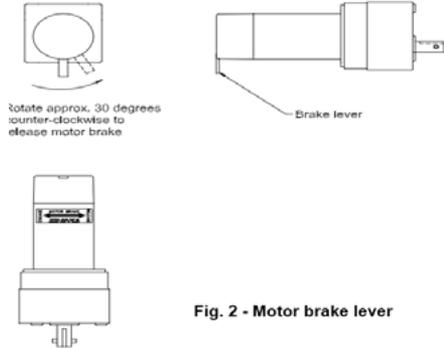
**Fig. 2 - Motor brake lever**
