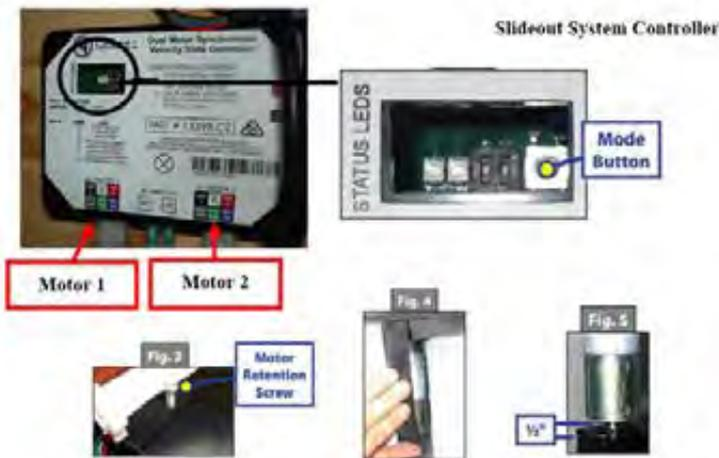
1. Locate the slideout system controller.
