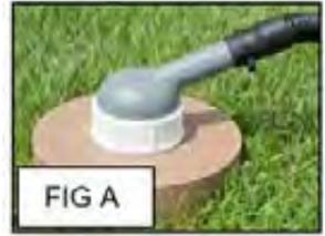
The **Macerator Bypass Valve** is located underneath the external hose storage box. This bypass will allow you to gravity dump the waste from the tanks straight down to a 3-inch sewer hose connection under the trailer, in the event there is a problem with the macerator motor.
