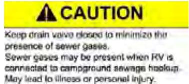
Some models are equipped with a side vent system. On these models this label will be next to the termination valve. This label should not be removed from your recreation vehicle.
