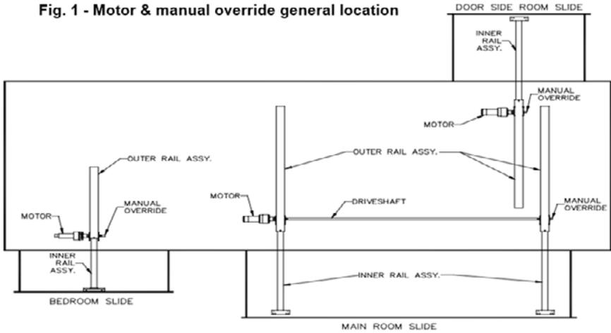
6. The room is now free to move. Using either a 5/8" or 3/4" wrench or socket, crank the room either in or out completely. If the slideout system is supplied with a gearbox override (optional), use the crank handle to move the room.
