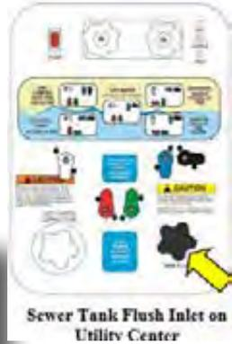
**NOTE:** The color-coded valve positions do not affect the tank flush function. It does not matter where they are positioned when operating the tank flush. Refer to the *Uni-Dock Utility Center*
