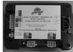
Fig.1 Slideout Controller
