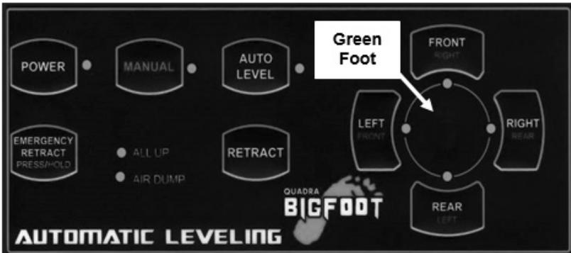
**NOTE:** When the unit is level, the green foot in the center of the right side switches will flash on and off.
