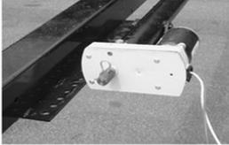
Fig. 3-Hex Head Crank Extension
