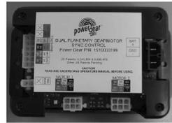
Fig.1 Slideout Controller
