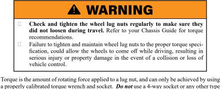
a properly calibrated torque wrench and socket. **Do not** use a 4-way socket or any other type of wrench that does not measure the actual pressure applied to the lug nut.
