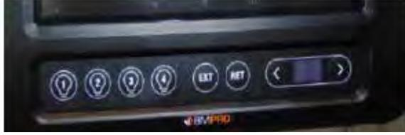
**NOTE:** Buttons #1 through #4 are pre-programmed from the factory and cannot be changed to perform other functions.
