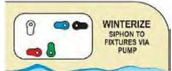
**NOTE:** When set to WINTERIZE: antifreeze will not enter the water heater or the fresh water tank. There are no dedicated water heater bypass valves.
