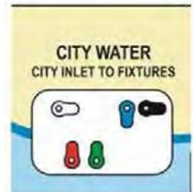
**To disconnect:** Turn off water at the pressurized source first, disconnect hose from the water source, (to release pressure off the system) then disconnect the hose at the city water connection on utility center last.
