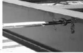
Fig. 2 - Through Frame Crank Extension w/Pin
