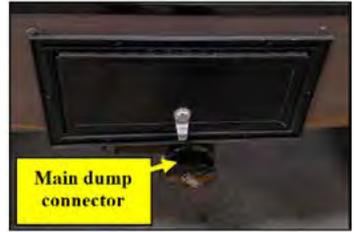
**NOTE:** The bypass valve also doubles as an emergency cutoff in the event of a problem with the flex hose or dump connector. Closing the valve stops waste flow out of the macerator pump and up to the flex hose, but will divert waste to the main dump connector under the RV. Make sure the main dump gate valve is closed until you are ready to empty the black tanks.
