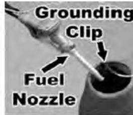
Fuel Nozzle in contact with receiving tank
