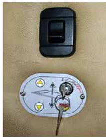
Fig.2 Key OFF (Vertical)
