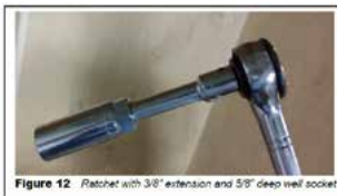
Figure 12 Ratchet with 3/8" extension and 5/8" deep well socket
