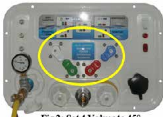
Fig 2: Set 4 Valves to 45°
