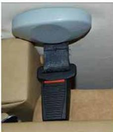
**Fig.1 Belt Interlock Latched**
