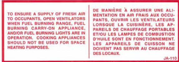
TO ENSURE A SUPPLY OF FRESH AIR TO OCCUPANTS, OPEN VENTILATORS WHEN FUEL BURNING RANGE, FUEL BURNING CARRY-ON APPLIANCE, AND/OR FUEL BURNING LIGHTS ARE IN OPERATION. COOKING APPLIANCES SHOULD NOT BE USED FOR SPACE HEATING PURPOSES.
