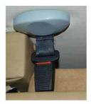
Fig.1 Belt Interlock Latched
