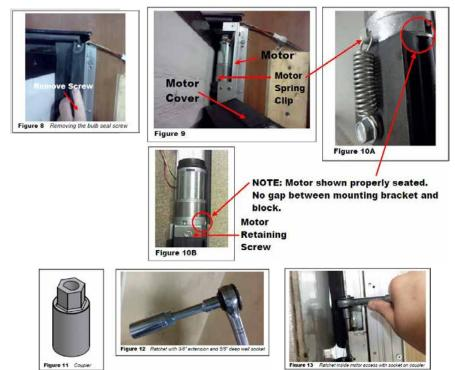
Power Gear Ram Slideout System
