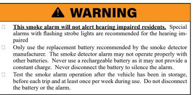
The smoke alarm is operational once the battery is correctly installed. It will not function if the battery is missing, disconnected, dead, the wrong type or not installed correctly. It requires one standard 9V battery. Refer to the user's guide, for correct battery and installation information,
