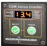
**<u>NOTE</u>**: When in *Inverter Mode* you will be able to cycle through Battery Voltage, Inverter Power, inverter settings and error codes. When in *Bypass Mode* you will be able to cycle through Battery Voltage, inverter settings and error codes. Inverter Power will not be available because the inverter is idle.
