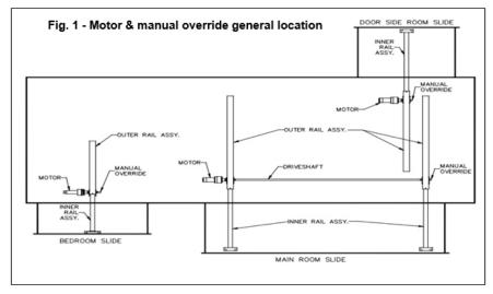
7. Locate the manual override for the slideout system (Fig. 1).
