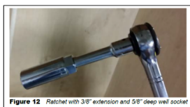
Figure 12 Ratchet with 3/8" extension and 5/8" deep well socket
