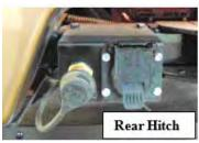
An air hose coupling (in the vicinity of the electrical harness connection) located at the rear of the motorhome supplies the air pressure to the tow vehicle controller.
