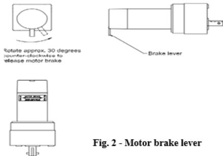
**Fig. 2 - Motor brake lever**
