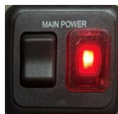
Battery Disconnect Switch
