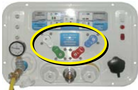
Fig 2: Set 4 Valves to 45°
