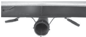
Black/Grey Tank Drain and Valves
